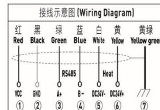
4-20mA current signal output: it is recommended to use RVVP/0.5mm<sup>2</sup> /copper core/low temperature resistant shielding cable, maximum communication distance is 1000m.
